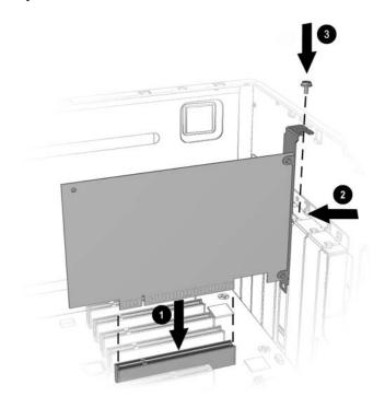
4. Place the slot screw **3** into the chassis slot and secure the expansion card to the chassis.
